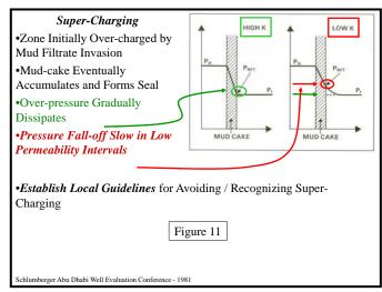
While unexpectedly high pressure points (Figure 10) can signal the presence of a permeability barrier, it's also possible that the measurement is reflecting *super-charging*: Figure 11.
