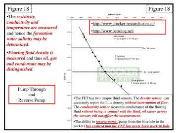
reversed, the additional ability to pump off the formation is available, should a tool sticking problem arise.
