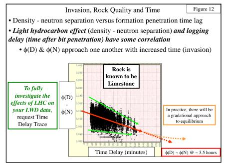
the Delta Porosity is displayed against Time Delay, as determined from the Drill Rate and LWD
