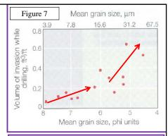
Volume of invasion in the first 15 minutes after drill bit penetration as a function of mean sand grain size, measured on core thin sections
