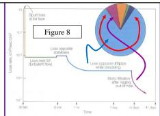
Filtrate loss rate into a permeable zone. The greatest fluid loss is during the Dynamic phase, when the drill pipe is opposite the zone of interest
