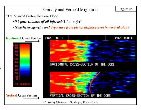
Calibrated CT-scans offer more than a simple visualization of the issue, and can in fact quantify the respective time lapse saturations (Figure 17).
