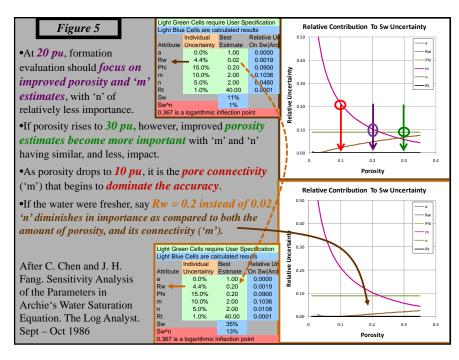
At 20 pu formation evaluation, with Chen's conditions, the focus should be on improved porosity and 'm' estimates, with 'n' of relatively less importance. If porosity rises to 30 pu, however, improved porosity estimates become more important with 'm' and 'n' having similar, and less, impact. As porosity drops below 20 pu, it is the pore connectivity ('m') that begins to dominate the accuracy: Figure 5.
