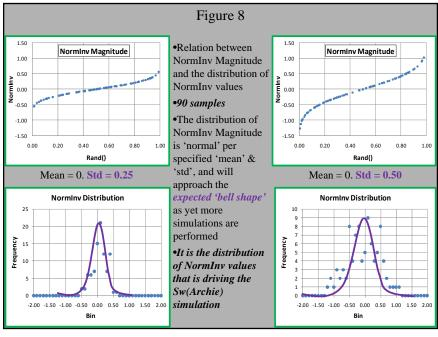
Figure 8 illustrates the relation between the random magnitude of NormInv, and the distribution of NormInv values, for different standard deviations, at 90 simulations. Both distributions take on an approximate Gaussian appearance, with the larger standard deviation result displaying more scatter. As the number of random calculations is increased, each distribution will approach the ideal Gaussian. It is the distribution of NormInv values that is driving the Sw(Archie)
