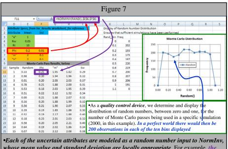
•Each of the uncertain attributes are modeled as a random number input to NormInv, whose mean value and standard deviation are locally appropriate. For example, the first pass random estimate of porosity, with a distribution centered on 20 pu and having a standard deviation of 1 pu, results in an estimate of 21 pu.
