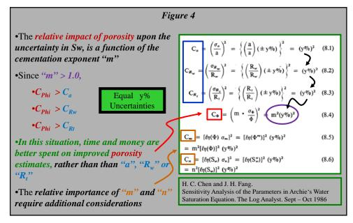
$C(\phi) > C(R_w)$ , C(a),  $C(R_t)$  simply because 'm' > 1: Figure 4. In such a situation, time and money are better spent on improved porosity estimates, rather than 'a',  $R_w$  or  $R_t$ .
