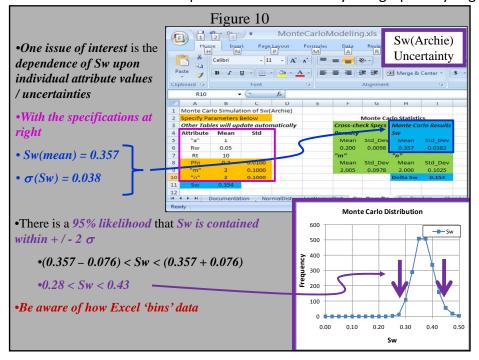
case, there is a 95% likelihood that Sw is contained within +/-2  $\sigma$ ,  $(0.357 - 0.076) < Sw < (0.357 + 0.076) <math>\Rightarrow$  0.28 < Sw < 0.43. The graphical display adds another dimension to the calculation.
