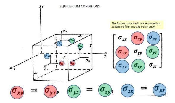
This permitted to simplify calculations of relations between stress and strain. Applying Hooke's law to the material under stress, mean to apply a 3x3 tensor multiplication to each elemental stress component for 3 faces of the elementary cube (resulting in a 3x3x3 tensor) and re-dimension (turn as vector rotation and change scalar value) to transform stress into the corresponding strain. For 3 faces of a cube a 3x3x3x3 tensor.
